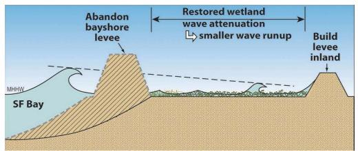
Figure 4- Retreat- Levee Relocation (Source: ESA-PWA, 2013)
