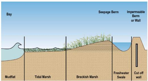
Figure 5- Horizontal Levee (Source: ESA-PWA, 2013)
